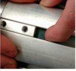
Insert the plate for the pressure connector.
