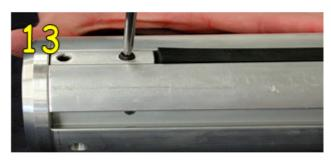
Without using too much force tighten the second grub screw of the locking plate around the pressure connector to ensure that it is air tight, with a no. 3 Allen key.
