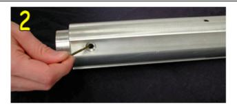
Grease the connecting hole of the valve.
