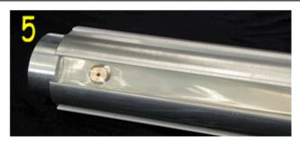
**K** Insert the bladder in the groove.
