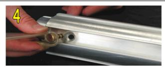
Insert the brass valve in the connecting hole of the valve.
