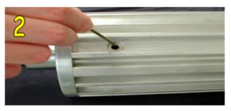
Grease the connecting hole of the valve.
