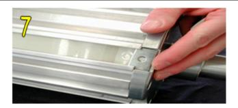
Insert the first closing plate of the bladder.
